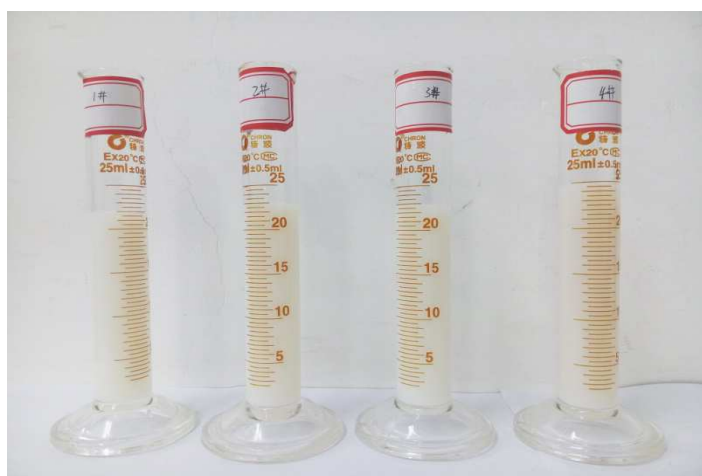
Fig 6 Nano paraffin emulsion after centrifugal
