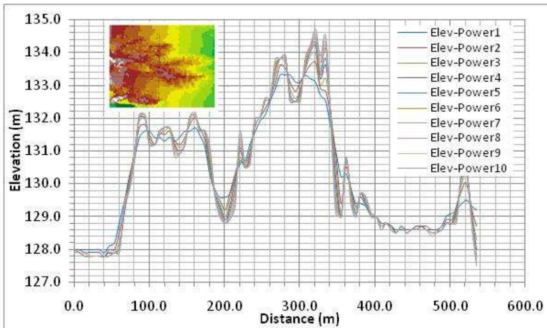
**Figure 12: Profile C-D in the DEMs created from spot elevation measurements using IDW of varying powers starting from power of one to the power of ten.**
