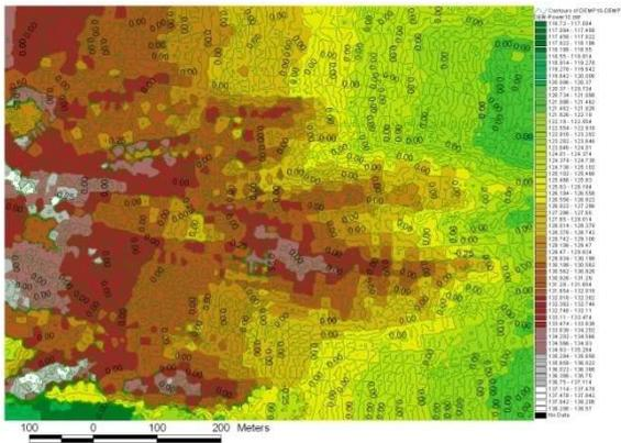
Figure 8: Contourlines generated from the differences between the DEM of power of ten and the DEM of power of seven.
