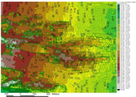
Figure 4: Contourlines generated from the differences between the DEM of power of ten and the DEM of power of three.
