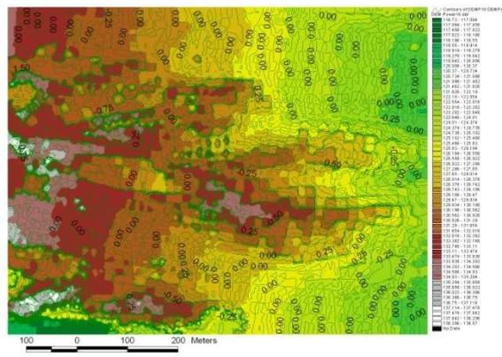
Figure 5: Contourlines generated from the differences between the DEM of power of ten and the DEM of power of four.
