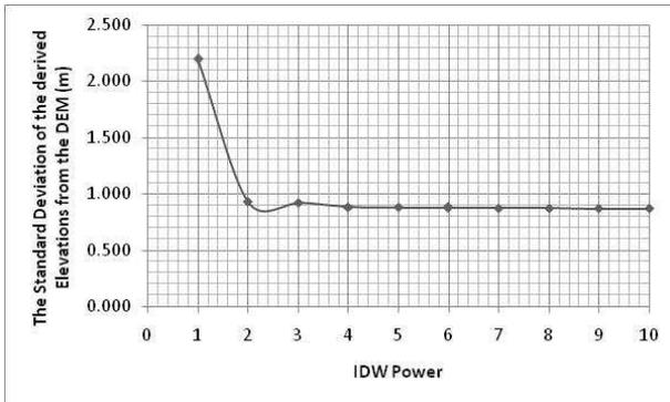
Figure 14: The sum of the residuals of the extracted elevations at the locations of the checkout points against the IDW power.
