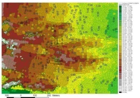
Figure 7: Contourlines generated from the differences between the DEM of power of ten and the DEM of power of six.
