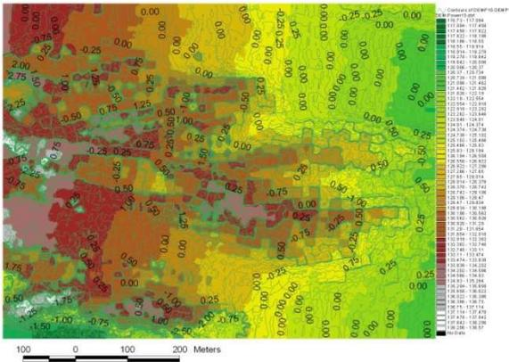
Figure 2: Contourlines generated from the differences between the DEM of power of ten and the DEM of power of one.
