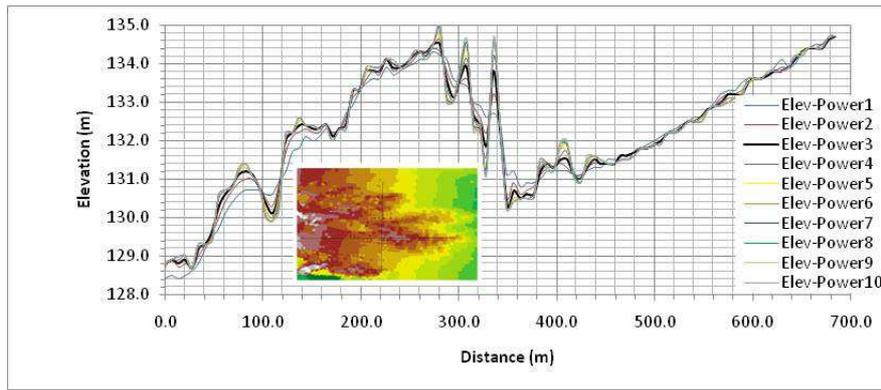
**Figure 11: Profile A-B in the DEMs created from spot elevation measurements using IDW of varying powers starting from power of one to the power of ten.**
