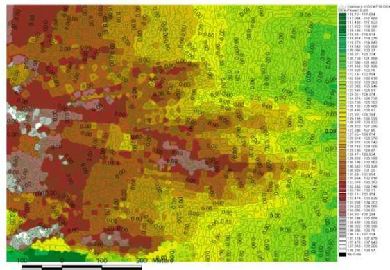
Figure 10: Contourlines generated from the differences between the DEM of power of ten and the DEM of power of nine.
