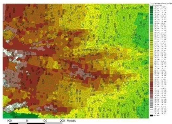
Figure 9: Contourlines generated from the differences between the DEM of power of ten and the DEM of power of eight.
