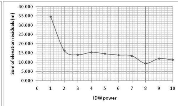
Figure 15: The standard deviation of the extracted elevations at the locations of the checkout points against the IDW power.
