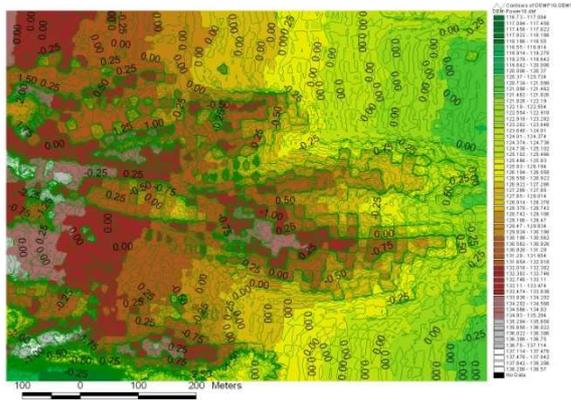
Figure 3: Contourlines generated from the differences between the DEM of power of ten and the DEM of power of two.
