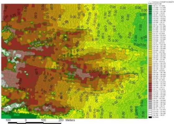
Figure 6: Contourlines generated from the differences between the DEM of power of ten and the DEM of power of five.
