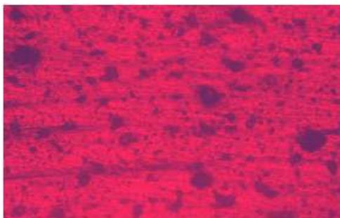
**Fig 9.** Sample Immersed in 0.2% inhibitor solution
